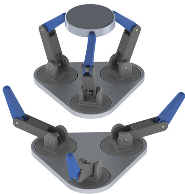
Fig. 1 When an open hand is closed to grasp an object, the kinematic structure is equivalent to a parallel robot
