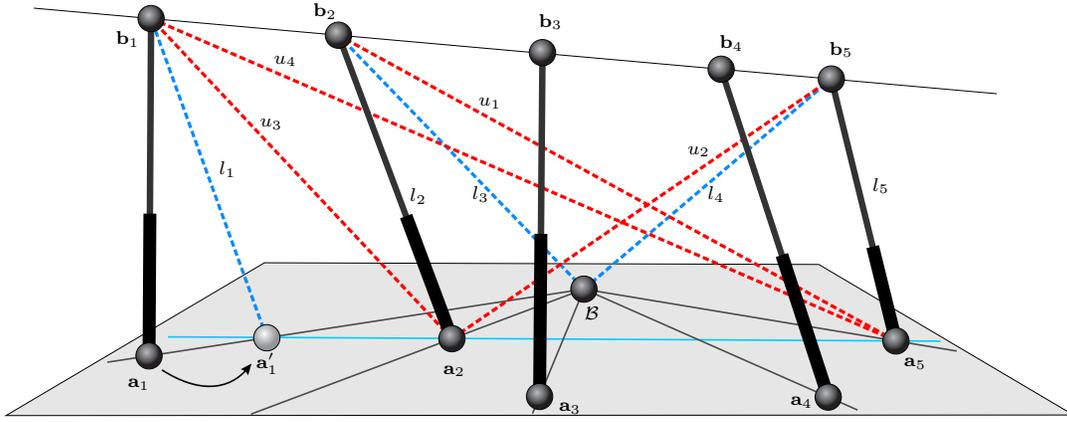
Fig. 7. The forward kinematics of a line-plane subassembly can be fully formulated in terms of distances.  $l_1$ ,  $l_3$  and  $l_4$  can be computed using the distance formula presented in Section V. Then,  $u_i$ , for  $i = 1, \dots, 4$  can be obtained using standard Distance Geometry techniques.
