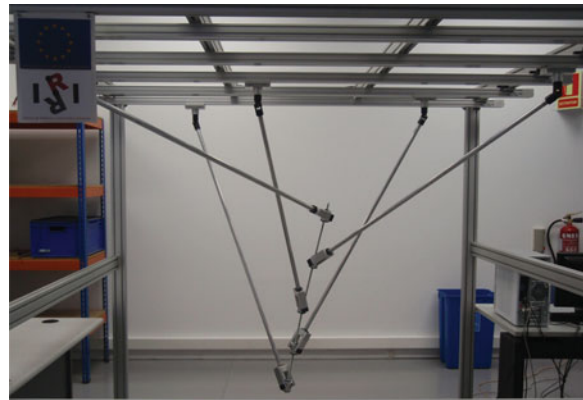
Fig. 7. Pentapod analyzed in Section V. Note that it is in an upside-down configuration, so that the platform is located under the base.
