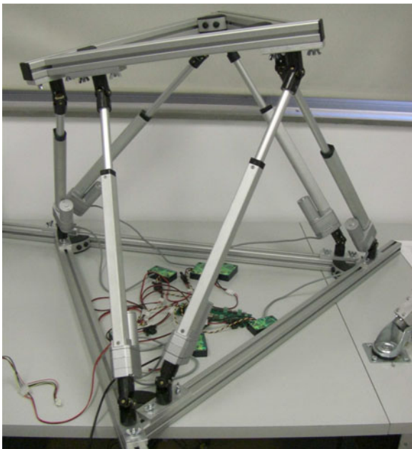
Fig. 6. This platform consists of six extensible legs connecting a moving platform to a fixed base. We avoid the use of multiple spherical joints (that is, spherical joints sharing the same center) without losing the properties of the celebrated octahedral architecture.
